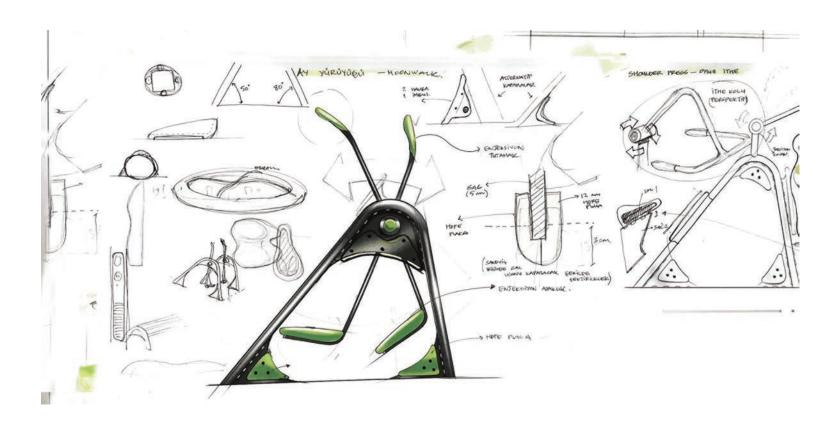
Ergonomic handles are made using plastic co injection with an elastomer cover. 55-shore elastomer provides a soft feel with UV resistance. 2-layer design has good grip and prevent sweating, making it easy for everyone to use them comfortably.
